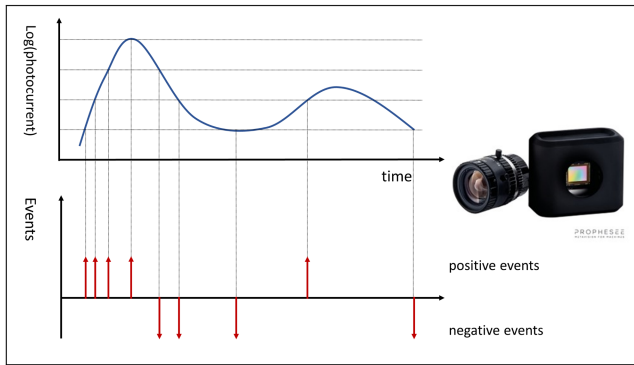
Fig. 1. The event-based camera from Prophesee [15] used in this work is shown. The intensity of the light is sampled by the camera, and an event is fired whenever the intensity exceeds by a certain value. Based on whether there is an increase or a decrease in the intensity, a positive or a negative signal is recorded.
