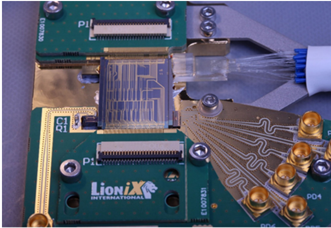
Fig. 8. Commercial example of TriPleX waveguide technology: Integrated Optical Beam Forming network showing hybrid integration of TriPleX and InP elements into an MWP module for satellite communications.
