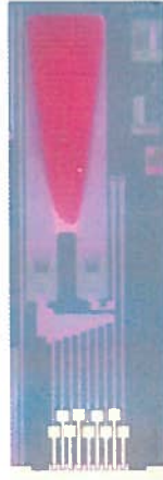
8 channel 2.3-2.4 um wavelength high resolution AWG spectrometer
