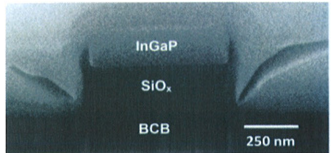
Fig. 3. A SEM cross-section of an InGaP waveguide with measured dimensions of 630 nm x 250 nm
