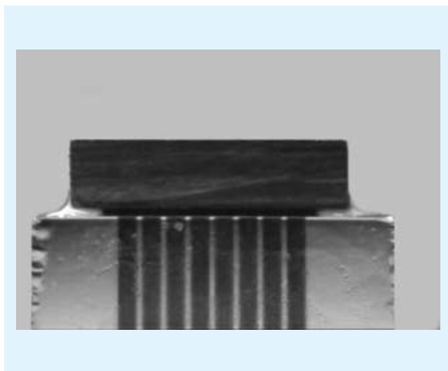
Figure 11. Photograph of the v-groove base with the mounted SOI die.
