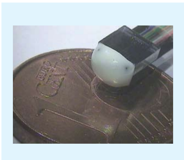
Figure 12. Photograph of the final fiber array package with glob-top protection. The solution is very compact due to the small scale of the nanophotonic die.
