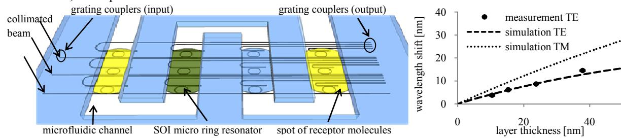
Fig. 1. A) illustration of the disposable lab-on-a-chip (not to scale), B) simulation and measurement of SiO<sub>2</sub> adlayers with increasing thickness.
