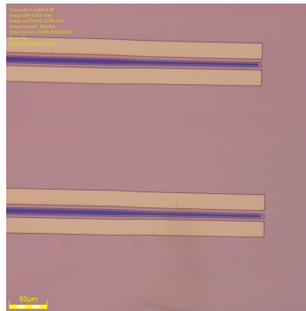
Figure 2.14: Microscope image of two laser mesa's after n-contact metallization.
