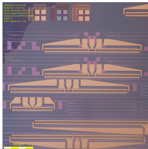
Figure 6.12: Microscope image of InAs/GaAs QD ring mode-locked lasers fabricated on a 400 nm SOI platform.
