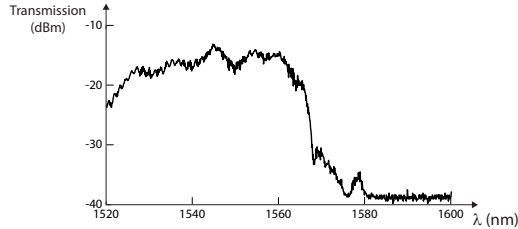
Figure 4.19: Upper band edge of an underetched bulk photonic crystal with a period a=580 nm and hole diameter d=0.6a , excited in the \Gamma M direction in air. Due to non linear buckling, the band edge is no longer sharply defined and it is difficult to use it as a measure for high resolution sensing.
